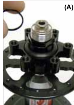
A. Some, but not all, hubs have a 1.5mm axle spacer.
