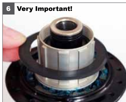
6. The large black Pawl Seal MUST be installed after the cassette body and axle have been joined with the hub shell. With the axle pushed completely into the hub shell and pawls engaged with the cassette body, install the large black pawl seal.
