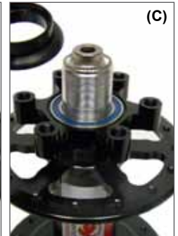
C. Remove spacer with attached dust seal.
