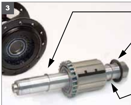
3. Separate cassette body and axle from the hub shell by grabbing the body and pulling out from the drive side.
