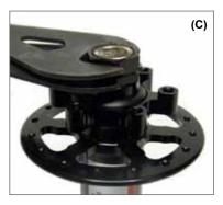
7. Grease the threads and install the new spacer with dust seal, install dust seal onto the adjusting nut and contuine. A) Finger tighten the adjusting nut with the shoulder side facing the hub shell (B) Install the lock nut and finger tighten (C) Using two 19mm cone wrenches, remove all play on adjusting nut, then back off one half rotation, 180 degrees.
