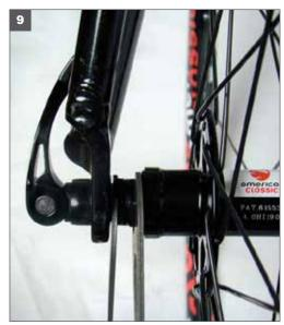
15. Hold the adjusting nut in place and loosen the lock nut. Slightly tighten or loosen the adjusting nut and hold in place. With the adjusting nut in place, tighten down the lock nut. Wiggle rim. Repeat Step 9 until the desired adjustment is acheived. Make sure the lock nut is tightened down when finished.
