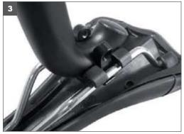
**Step 3:** Press the top of the seatpost down into position while sliding the 2 lower clamp pieces into place.
