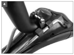
**Step 4:** While holding the lower clamp pieces in place, install the 4mm hex bolt (lightly greased). Do not tighten completely.
