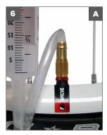
A. Recommended: Attached sealant injector to valve, pinch injector tube, pour sealant into injector, release tube and push plunger.
