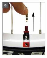
After air has been let out of tire and beads are still seated, unthread and remove valve core.
