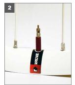
2. Insert red valve stem with rubber O-ring into the tire well
