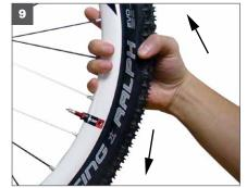
9. Once the beads are seated and the tire is holding air with sealant inside, you will need to shake the wheel evenly to spread the sealant in the tire until any small air leaks are sealed. Shake in many directions.
