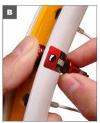
B. Firmly press valve base into rim with your thumb and finger tighten knurled nut.
