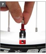
7. Reinstall the valve core. Hand tighten only, do <u>not</u> use a wrench or pliers.
