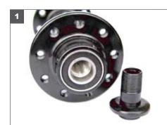
Using two 5mm hex wrenches, hold one end cap while turning the other counter clockwise. This will remove only one end cap. Continue to Step 2.
