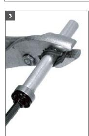
The second cap is still attached to the axle along with the second bearing. Grab the axle firmly with a set of pliers. Unscrew the cap and the bearing will be be free. Slight scuffing of the axle by the pliers is okay. The axle sleeve does not rotate when the wheel turns.
