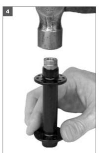
Position a new bearing onto the hub shell. Place one of the old bearings on top of the new bearing (to protect it) and gently tap in the bearing. Flip the hub over and insert the axle into the open end of the hub shell. Install the second bearing. Damage can occur to the hub shell if bearing are not intalled straight.
