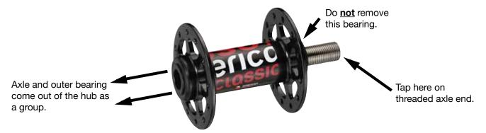
**STEP 1B.** The new axle includes a bearing, you may throw out the fixed axle and used bearing. Go to STEP 3.
