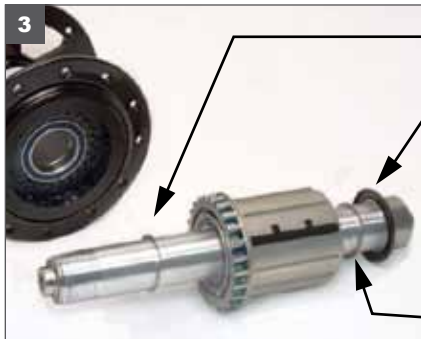
1. Using two 19mm cone wrenches, loosen the lock and adjusting nut. 2. Remove lock nut. A. Some, but not all, hubs have a 1.5mm axle spacer. B. Remove adjuster nut. C. Remove spacer with dust seal. Hubs with serial numbers beginning with "D" or "E" or ending with "III" do not have this spacer.
