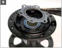
9. With a thin layer of clean grease coating the hub shell, install the cam plate. Refer to the picture for the correct orientation. Do not put the cam plate in upside down.
