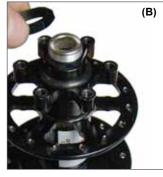
(B) Install the lock nut and finger tighten **-OR-** if you have a serial number beginning with "D" or "E" or ending with "III" re-use your 6.5mm lock nut or 1.5mm spacer.
