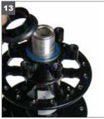
13. Grease the threads and install the spacer with dust seal. Hubs with serial numbers beginning with "D" or "E" or ending with "III" will not have this spacer.
