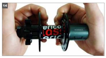
14. Holding the wheel by the hub flanges, use your palms to check if the axle moves side-to-side. If the axle moves side-to-side, tighten the lock and adjusting nuts slightly until it does not move side-to-side. When finished, the axle and cassette body should spin freely.
