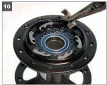
10. With a thin layer of clean grease coating the top of the cam plate, install all 6 pawls. Once completed the pawls should freely engage in unison with the cam plate.
