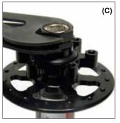
(C) Using two 19mm cone wrenches, remove all play on adjusting nut, then back off one half rotation, 180 degrees.
