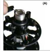
(A) Finger tighten the adjusting nut with the shoulder side facing the hub shell. For hubs with serial numbers beginning with "D" or "E" or ending with "III" install the dust seal on the adjusting nut.
