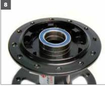
**8. Bearing Installation:** Position a new bearing onto the hub shell. Place old bearing on top of new bearing.
