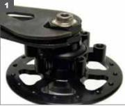
1. Using two 19mm cone wrenches, loosen the lock and adjusting nut.
