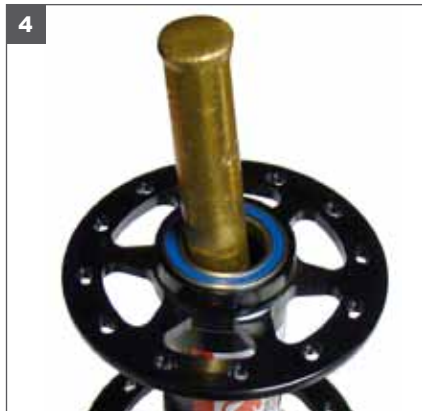
4. Insert a punch through the hub and rest on inner race of the opposite side bearing. Tap punch in a circular motion with a hammer around inner race to remove bearing. Flip hub over and repeat to remove second bearing.
