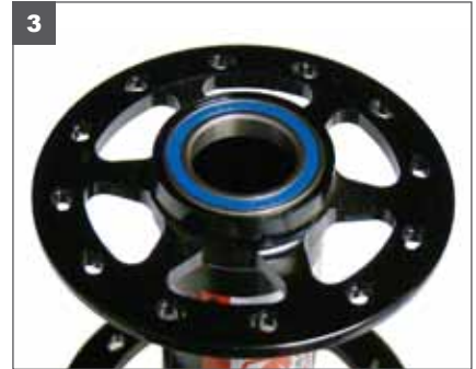
3. Hub shell with 6803-C3 bearing. There is one bearing on each side of the hub.
