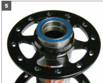
5. Position a new bearing onto the hub shell. Place one of the old bearings on top of the new bearing and gently tap in the bearing. Flip the hub over and repeat to install second bearing. NOTE: Damage can occur to the hub shell if bearings are not installed straight.
