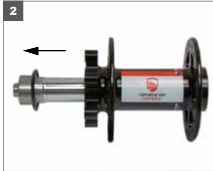
2. Push the quick release axle to the disc side, and pull the axle from the hub.
