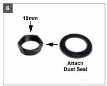
6. Insert the dust seal in the groove on the outside of the 19mm adjusting nut.
