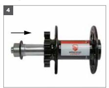
4. Insert the 9mm quick release axle from the disc side of the hub.
