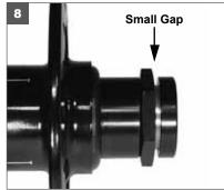
8. Thread endcap fully onto axle. NOTE: The end cap will **NOT** tighten onto the adjusting nut. There will be a small gap between the end cap and adjusting nut. There is an O-Ring in the adjusting nut so it does not need to be locked down.
