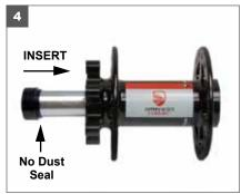
4. Insert the BOOST 15mm x 110mm thru axle from the disc side of the hub. Dust Seal is installed in Step 9.
