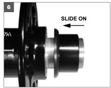
6. Slide 10mm Spacer with Dust Seal on to the end of the BOOST Thru Axle.
