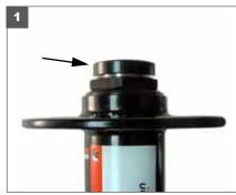
1. Holding the opposite end of the axle end cap stationary, unthread the non-disc side end cap.
