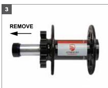
3. Push the 15mm thru axle to the disc side, and pull the axle from the hub.
