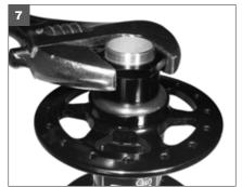
7. Thread the 22mm Adjusting Nut onto the end of the 10mm Spacer and tighten with a wrench. Tighten the adjusting nut until there is no play and back off one quarter rotation.
