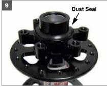
9. Finally slide the remaining dust seal over the end cap on the disc side.
