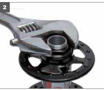
2. Using a 22mm wrench, turn counter clockwise to loosen and remove the 22mm Adjusting Nut.
