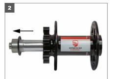
2. Push the quick release axle to the disc side, and pull the axle from the hub.
