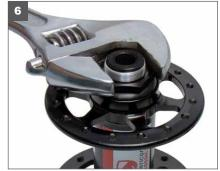
6. Thread the 22mm adjusting nut with dust seal attached onto the end of the 9mm thruaxle and tighten with a wrench. Tighten the adjusting nut until there is no play and back off one quarter rotation.
