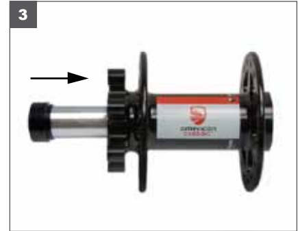
3. Insert the 15mm thru-axle from the disc side of the hub.
