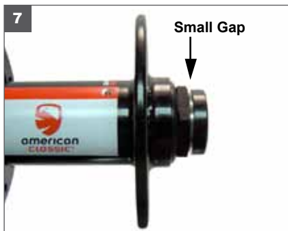
7. Thread endcap fully onto axle. NOTE: The end cap will NOT tighten onto the adjusting nut. There will be a small gap between the end cap and adjusting nut. There is an O-Ring in the adjusting nut so it does not need to be locked down.
