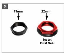
5. Insert the dust seal in the groove on the outside of the 22mm Adjusting Nut.
