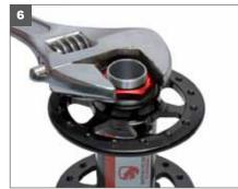
6. Thread the 22mm Adjusting Nut with dust seal attached onto the end of the 12mm Thru Axle and tighten with a wrench. Tighten the adjusting nut until there is no play and back off one quarter rotation.
