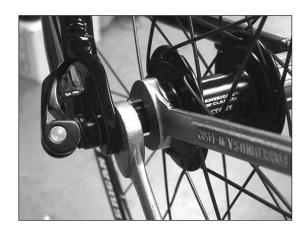
Hold the adjuster nut and loosen the lock nut. Tighten the adjuster nut. Hold the adjuster nut and tighten the lock nut. Fix dust seal if needed.
