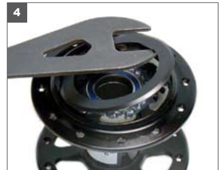
3. Separate cassette body and axle from the hub shell by grabbing the body and pulling out from the drive side. 4. Remove large black pawl seal.
