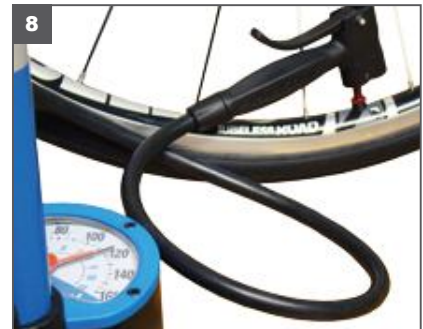
8. With the valve core installed, pump air back into the tire and seat the tire beads.
