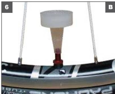
B. Sealant bottles often come with a funnel style cone cap that can be used if you do not have an injector.
