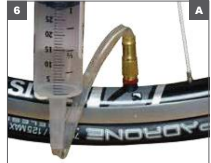
A. Recommended: Attached sealant injector to valve, pinch injector tube, pour sealant into injector, release tube and push plunger.
