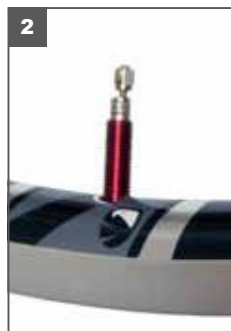
2. Insert red valve stem with rubber O-ring into the tire well.
