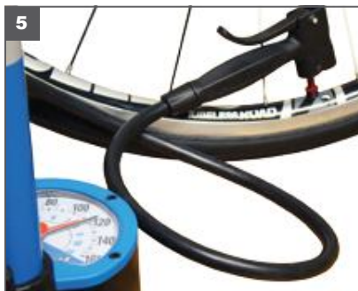
5. After the beads catch, finish inflating the tire. Do not exceed the manufacturer's maximum air pressure rating. (PSI/Bar)
