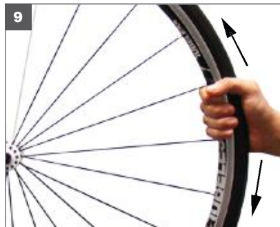
9. Once the beads are seated and the tire is holding air with sealant inside, you will need to shake the wheel evenly to spread the sealant in the tire until any small air leaks are sealed. Shake in many directions.
