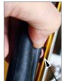
B. Firmly press valve base into rim with your thumb and finger tighten knurled nut.
