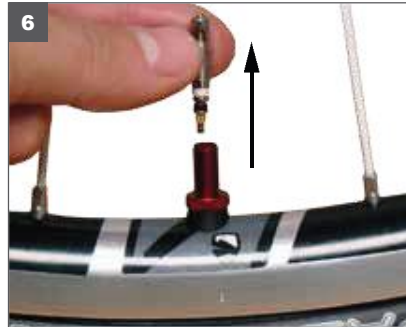
6. After air has been let out of tire and beads are still seated, unthread and remove valve core.
