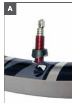
A. Use the plastic contoured spacer to protect the rim from the nut.
