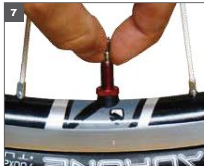
7. Reinstall the valve core. Hand tighten only, do not use a wrench or pliers.
