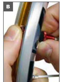
B. Firmly press valve base into rim with your thumb and finger tighten knurled nut.
