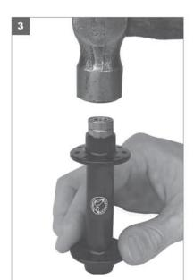
Position a new bearing onto the hub shell. Place one of the old bearings on top of the new bearing (to protect it) and gently tap in the bearing. Damage can occur to the hub shell if bearings are not installed straight.
