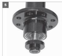
The new bearings are installed correctly if they are slightly recessed in the hub shell as shown in the picture. By using the old bearings during installation, the new bearings should be in the correct position. The axle inside should not be loose. Insert the end caps into each end of the axle. Congratulations, you are finished.
