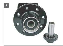
Remove both end caps using a pair of long nose pliers. Place one tip of the pliers directly into the end cap (where the skewer goes) and place the other tip on the outside (where the fork ends sit). Gently squeeze and pull out.
