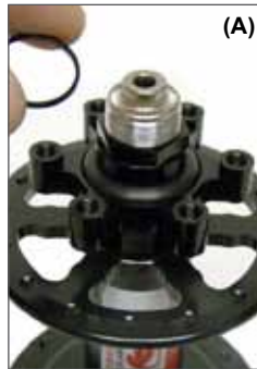
A. Some hubs have a 1.5mm axle spacer.
