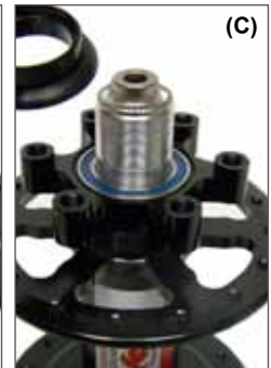
C. Remove spacer with attached dust seal.
