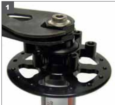
1. Using two 19mm cone wrenches, loosen the lock and adjusting nut.
