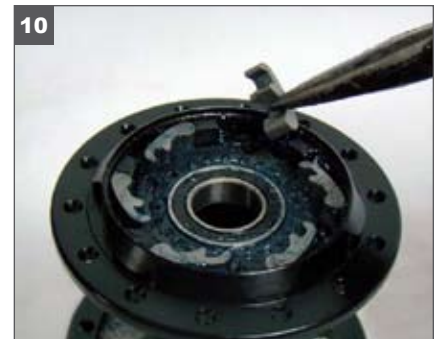
10. With a thin layer of clean grease coating the top of the cam plate, install all 6 pawls. Once completed the pawls should freely engage in unison with the cam plate.
