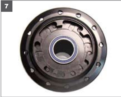
7. Clean out the hub shell for inspection and new grease.
