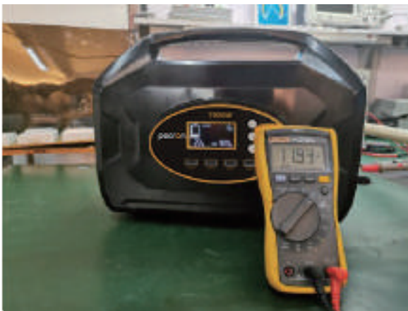
7.2.3 12V DC output test
