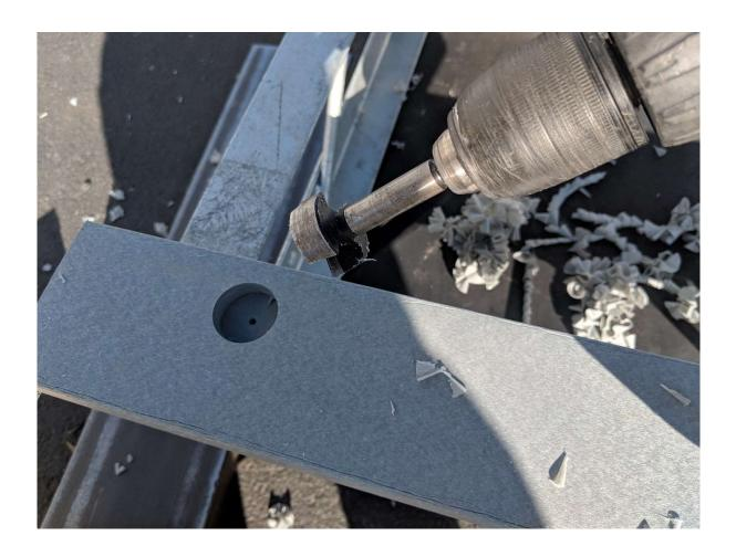
Once you drill with the paddle bit, finish hole by using a  $\frac{1}{2}$ " drill bit all the way through.
