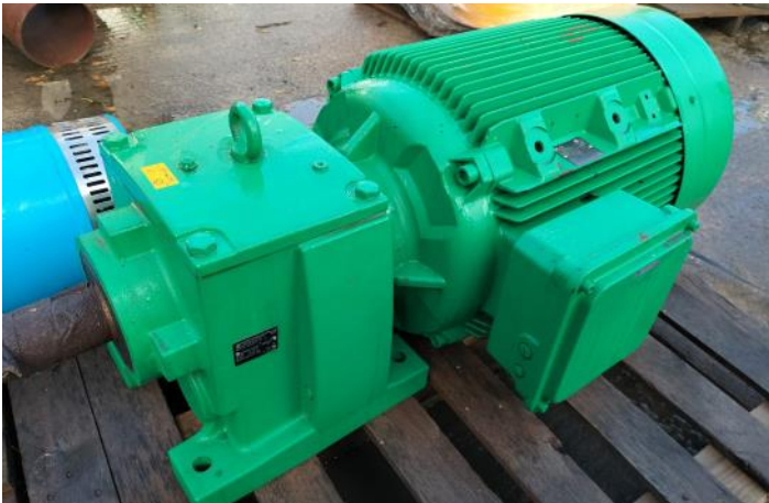
Nord Motor / Gearbox
