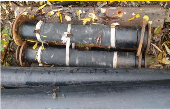
5" Wire Armoured 1m Spools c/w Swivel Flanges
