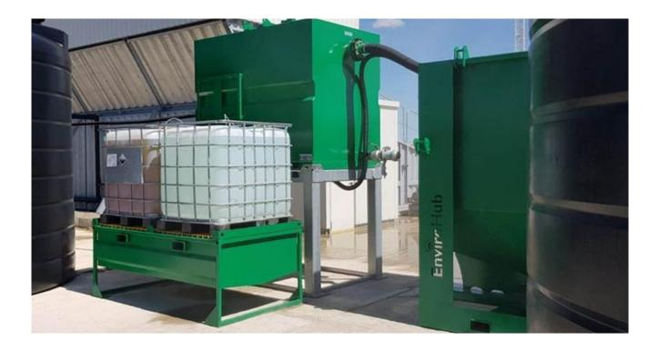
EnviroHub is a control system used by the quarrying and construction industries to monitor, treat and report on water quality onsite.
