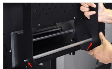
Step 18. Before installing the number 2 bracket, insert the press bar into the pre-made hole positions.
