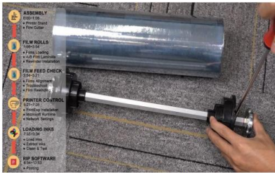
Step 1. Now we start the film rolls installation. First get the plastic holder of one side off.
