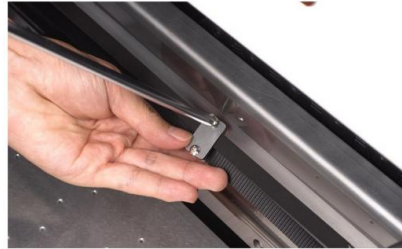
Step 22. Loose the screws and get the plates removed. If a printer works with the plates on the belt, the belt may get deformed.
