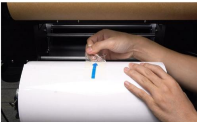
Step 35. Now we load A film in. Pay attention to the direction of the film leading edge.
