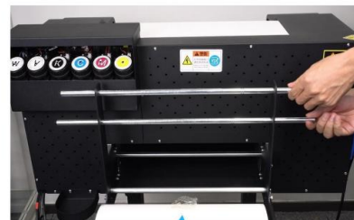
Step 30. Now insert two bars. These 2 bars are for the film rewriter.
