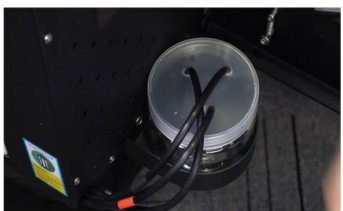
Step 23. Extract 5 to 10 millimeters of ink out of each labeled tube, then put the tubes back to its place.
