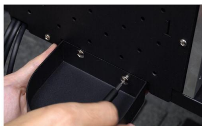
Step 19. Get the screws back and fasten them.
