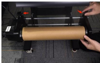
Step 5. And twist the knobs to fasten the position of the rewriter.
