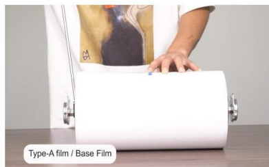
Step 9. The installation procedures are quite the same. One important point is to keep the 2 bearings symmetrical and the A film roll in the middle.
