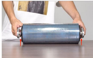
Step 6. Make the 2 bearings symmetrical on both sides and keep the film roll centered.
