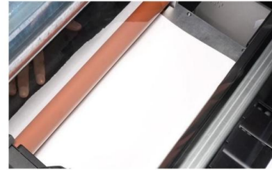
Step 38. There is a sticky adhesive layer on the base film, watch out not to stick it with any parts of the printer.
