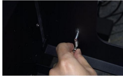
Step 26. But loosely twist the Hex screw onto the bracket, no need to secure it tightly.
