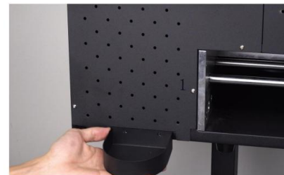
Step 18. Install a tray for ink waste bottle.
