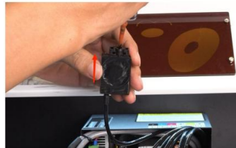
Step 12. Don't turn the ink cartridge downward when extracting ink, this will cause many bubbles in the ink. Always hold a cartridge UPWARD.
