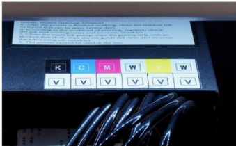
Step 15. Go on extracting from all the cartridges. Pay attention to the positions of color ink cartridges. For example, these 2 white inks are separated by yellow.
