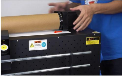
Step 31. Insert the cardboard tube onto the rewinder. The protective film on the Type-A film will be wound onto the cardboard tube.
