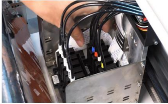
Step 11. Don't take off all the ink cartridges at the same time. Some ink cartridges are interconnected, air will enter other ink tubes.
