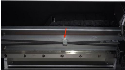
Step 21. Here we notice a metal fixing plate, it secures the drive belt during transportation.
