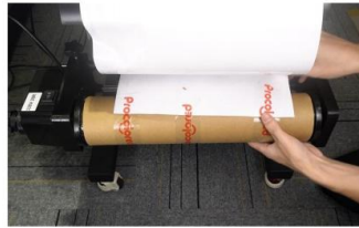
Step 6. Use some adhesive tape to secure the leading edge of the laminated film.
