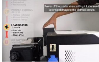
Step 2. The ink tank locates at the right back of the printer.
