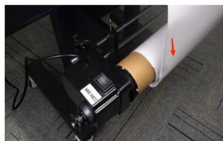
Step 10. We can see the laminated films can be rolled up automatically. If it doesn't, adjust the torque
