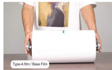
Step 8. Now we go on to install A film, also called base film in UV DTF printing.
