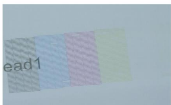
Step 25. If there are too many broken lines, press the clean button to clean the print-head.
