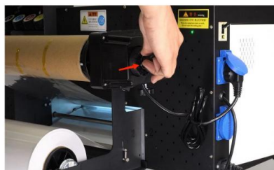
Step 18. Twist the adjustment knob to increase rolling torque. Make sure the device provides the very appropriate torque to tighten the retracted protective film.
