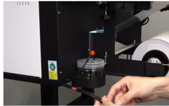
Step 20. The printer comes with 3 waste ink tubes. ① The one without labels for waste ink that dropped off from the print-head parking position.
