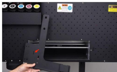
Step 15. Now we install brackets for Type-A film roll. First get the bracket marked with number 1.
