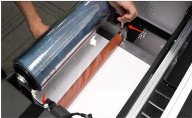
Step 11. Both ends of the heating roller need to maintain the same tension to prevent the base film from gradually deviating.
