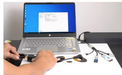
Step 29. If you are not sure which network is from the printer, you can unplug and reconnect the data cable of the printer. The printer Ethernet will pop up again.
