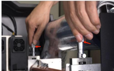
Step 12. Rotate the two thumb screws to set the tension.
