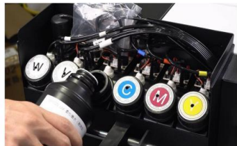
Step 7. Add corresponding inks into these containers. If you pour the fault ink into a tank, you need to empty the ink from the tank with syringe and ink pumping tube.
