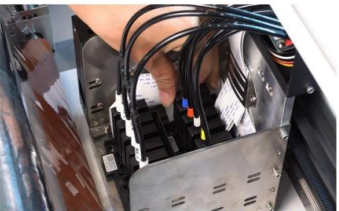
Step 13. Take off only one cartridge at a time and turn it upward to extract 5 to 10 millimeters of ink until the cartridge is free of air. And gently put it back after extracting.
