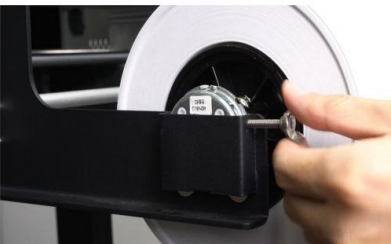
Step 29. Use 2 wing screws to secure the bearings on both sides of the film roll.
