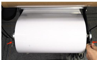
Step 7. We need to check whether the wing screws have secured the roller bearings.
