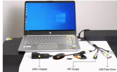
Step 2. Besides USB drive, there is also a blue RIP dongle, it's needed every time you use the RIP software. And we also have a USB 3 adapter for you. It is capable of fast data transfer. If the WAN port of your computer reach a speed of 1 Gigabit per second, you don't need this USB adapter.
