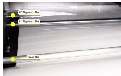
Step 36. Guide the film sheet to go under the press bar and the first alignment bar and go over the second alignment bar.
