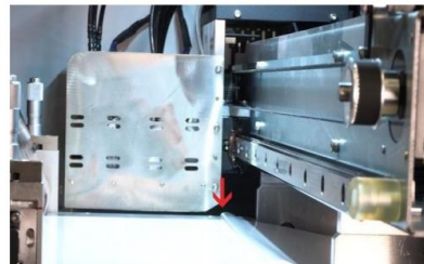
Step 16. In this case, the protective film is not automatically retracted. That means the film rewinder doesn't provide enough torque.
