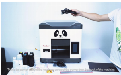
Step 3. This is the power cord of the machine, connect the power from the back of the machine.
