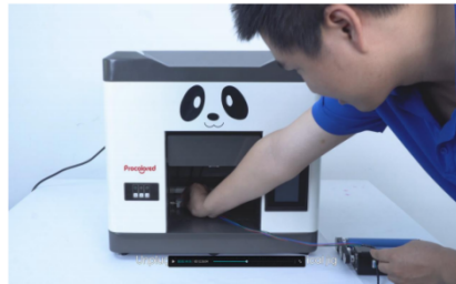
Step 2. Connect the Jig plug to the printer
