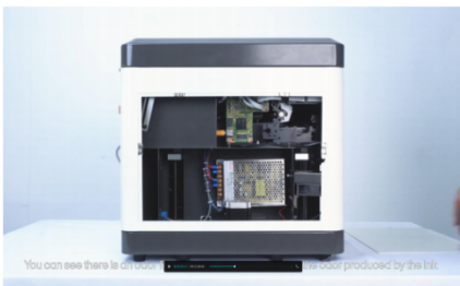
Step 13. Open the left side cover
