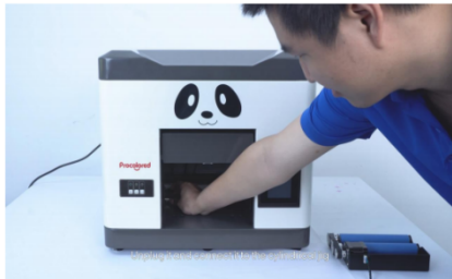
Step 1. Unplug the connection plug under the platform
