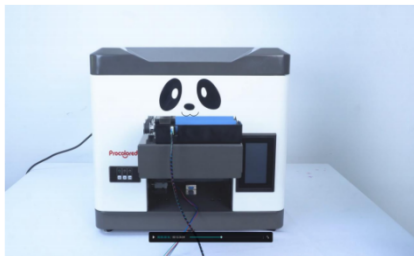
Step 3. Place the cylindrical jig on the printer platform
