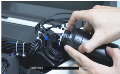
Step 1. Pour ink to the bottle in according to color sequence
