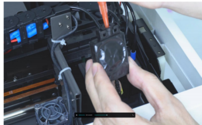
Step 2. Pull ink out from the damper
