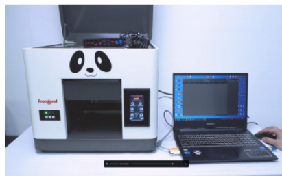
Step 4. Clean the print head in software
