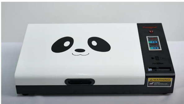
Step 3. Powder curing will be done by an oven like this. Set the temperature at 120 degrees Celsius and the countdown timer to 150 seconds. The curing time is flexible, if the print is too wet, it need longer time to dry up entirely.
