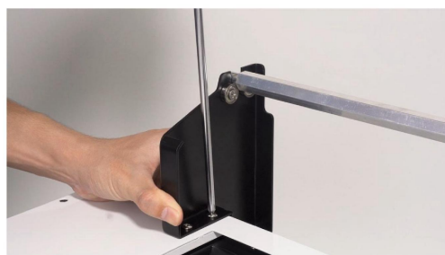
Step 10. Once the bracket position is confirmed, tighten the screws fully this time.
