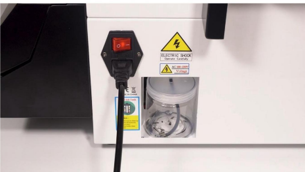
Step 45. And put the waste ink bottle back too.
