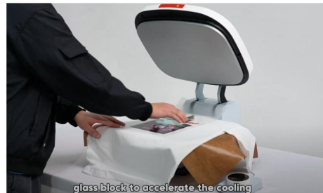
Step 6. It's recommended to use a glass block to accelerate the cooling, as cold peeling allows better transfer of the design onto the fabric.
