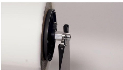
Step 19. Ensure the film roll can rotate smoothly on the brackets.
