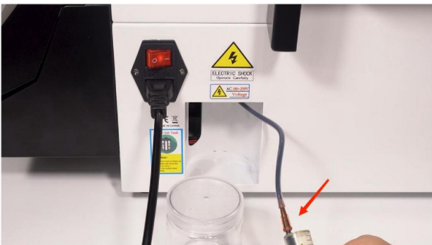
Step 43. Extract 5 to 10 milliliters of ink out of the waste ink tube.
