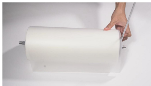
Step 16. Once the position is confirmed, secure the screws on the plastic holder.
