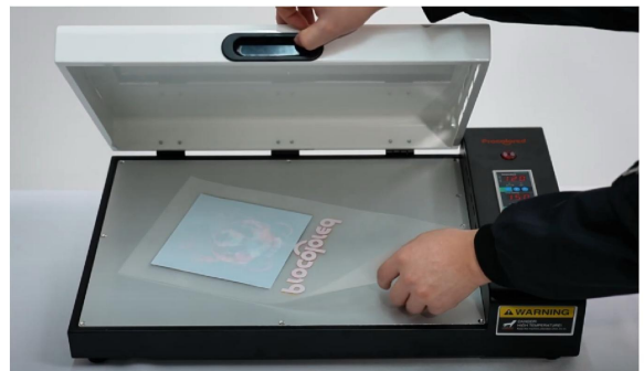
Step 4. Printing film face down, gently put the film on the oven pad.
