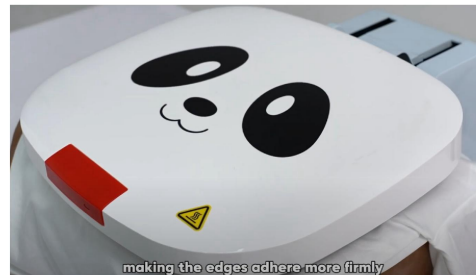
Step 8. Third heat press for 10 seconds to secure the print, making the edges adhere more firmly to the fabric and prevent edge lifting.
