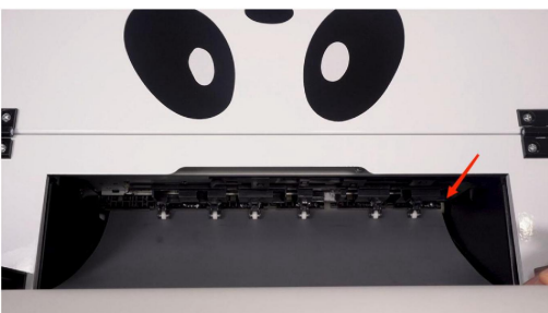
Step 29. Make sure the film goes straight.
