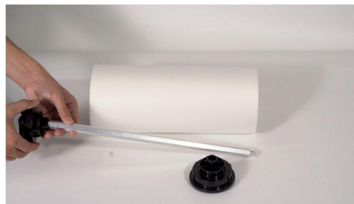
Step 12. Fetch the roller down and slide the plastic holder onto it.
