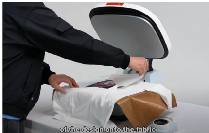
Step 7. And now you can peel off the film! Make sure to do the peeling gently and slowly.
