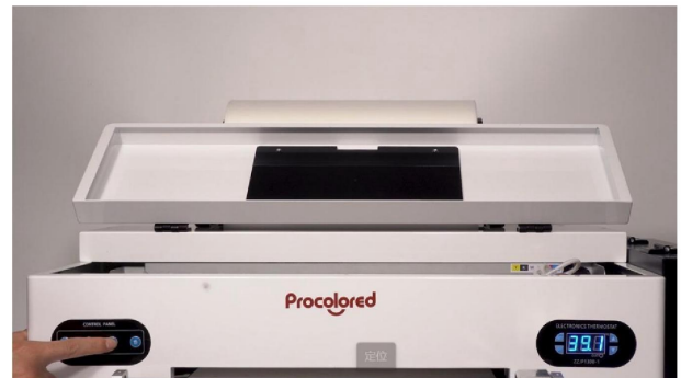
Step 46. Long press the ink button to execute print head cleaning. [the left third button]
