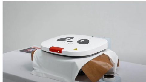
Step 2. The transfer process requires three separate heat presses. First heat press for 10 seconds at 160°C/320°F to keep the garment flat.
