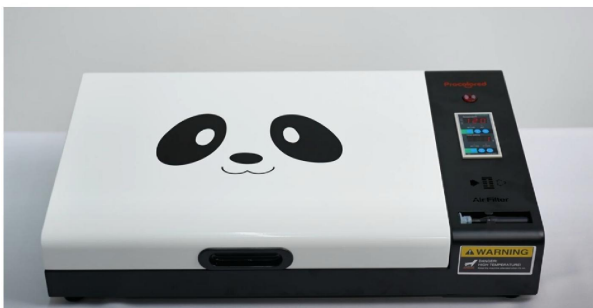
Step 5. Press start and wait for the curing. In the oven, adhesive powder is melting down, inks are curing/drying up and embedding onto the adhesive layer.
