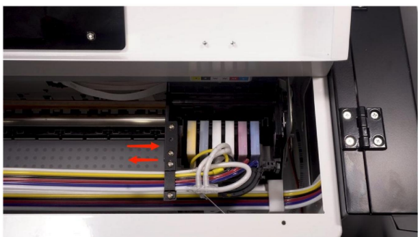
Step 47. The print head will move back and forth automatically to finish the cleaning which takes about 2 minutes.
