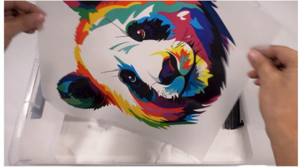
Step 2. Before curing, don't forget to shake the film slightly to remove the spare powder.
