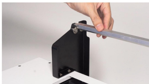
Step 9. Rotate the roller to check if the bracket distance is appropriate and safe.
