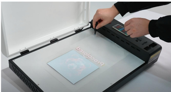
Step 7. We highly recommend to use a suction cup to fetch the cured printing film, since the oven pad and film might be really hot.
