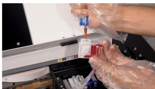
Step 38. Turn it upward to extract 5 to 10ml of ink until there is no much air in the cartridge.
