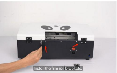
Step 5. Now we install the two brackets at the rear. Load the brackets and fasten the screws at both sides.
