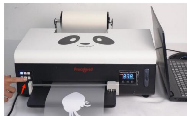
Step 7. When the printing is done, press the bottom middle button to load more film.
