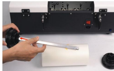
Step 6. Insert the roller bar into the plastic holder.
