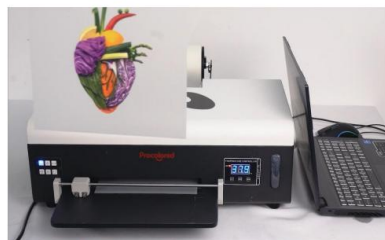
Step 9. The DTF printing has done! To apply this on your shirt, you'll need to do more processing like powdering, curing and heat press. Please search for more Procolored videos online for related information.
