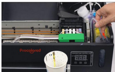
Step 9. Pull out the ink tube in the waste ink bottle.
