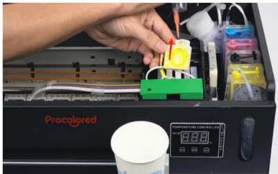
Step 6. Take only one ink cartridge out at a time and always hold it upward.
