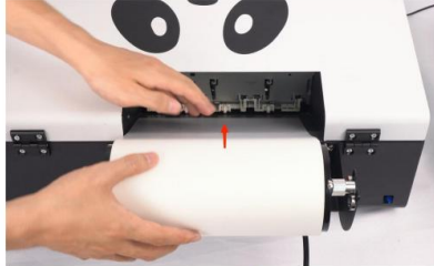
Step 12. Load the film into the printer (the side with coating facing up).
