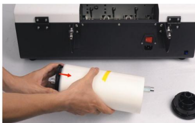
Step 7. Insert the film roll into the roller bar, remember to push the film to the left end.
