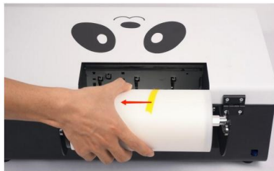
Step 10. Load the film onto the printer, place the film roll to the farthest left [the left when we're facing the rear of the printer].
