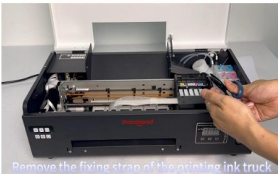
Remove the fixing strap of the printing ink truck
