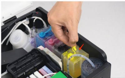
Step 5. Now we're going to extract some inks out of the ink cartridges. First remove all rubber lids of the vent holes.
