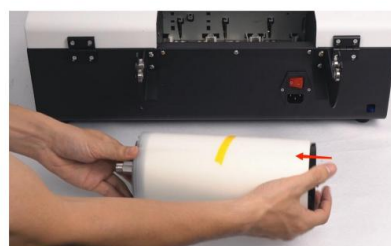
Step 8. Insert the other plastic holder in, also, push it to the end.
