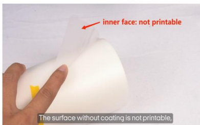
Step 9. Before loading the film on the printer, do pay attention to the correct side of the film - film without coating [the inner side] is not for printing.
