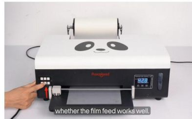
Step 16. Press the bottom middle button, to test if the film can be loaded smoothly.
