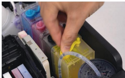
Step 4. After finishing adding, put the rubber lid back.
