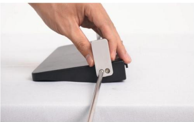
Step 3. Fasten the screws of the other side.
