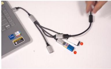
Step 1. Insert the blue dongle and USB drive (we highly recommend to use a USB splitter to perform simultaneous operations more conveniently).
