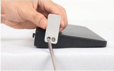
Step 1. Fasten the side screws of the film exit plate.
