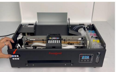
After completion, please move the printing ink cart to the middle position
