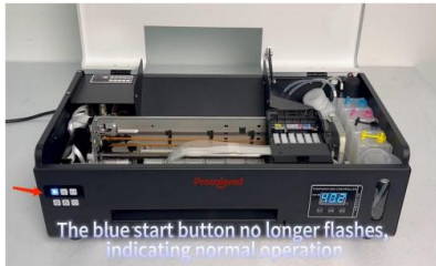
Step 13. This test might take a little longer time and it will finish when the first button stops flashing,
