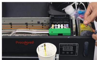
Step 10. Also extract 5ml waste ink out. After all the extracting, don't forget to put all the rubber lids of the vent holes back.
