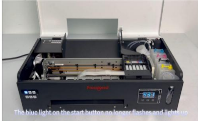
Step 11. When the self-test finishes, the first button will no longer flashes.
