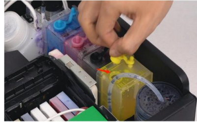
Step 2. Remove the rubber lid of the ink hole in the ink tank.
