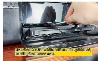
Step 27. Use swabs to clean the print head bottom.
