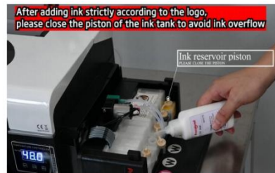
Step 16. Put the piston back in place after every ink-adding.
