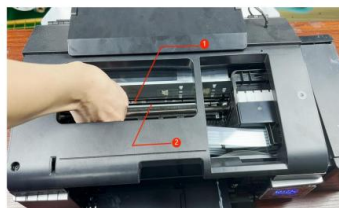
Step 15. We now need to gently clean ①encoder strip and ②printer belt with the lint-free cloth. They're supposed to be cleaned every 7 days.
