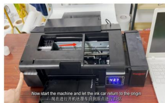
Step 28. After the cleaning, press the switch button to set the print head assembly back to the farthest right.
