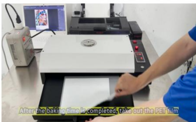
Step 19. When the curing is over, carefully fetch the hot cured film.
