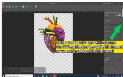
Step 6. L805 DTF has two white ink channels, so here we need to click + icon to add one more white channel.
