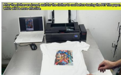
Step 25. When the heat pressing is done, wait until the printing has cooled down, then gently peel off the film.
