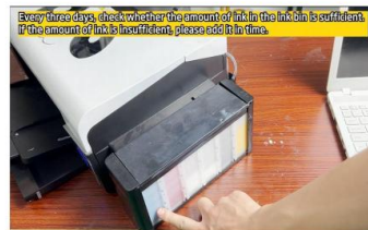
Step 30. Besides above daily maintenance, it's also recommended to occasionally check if there's enough ink left.
