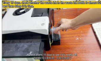
Step 31. Also, from time to time, check the waste ink bottle, empty or change it if needed.
