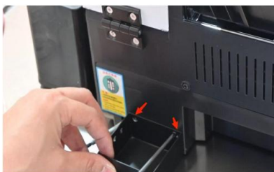
Step 3. Install the waste ink bottle tray on and fasten the screws.
