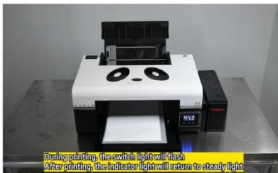
Step 13. The switch button will keep flashing till the printing task is finished.
