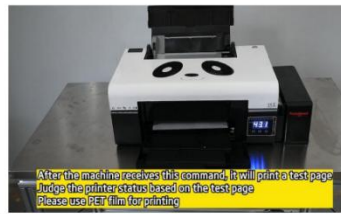
Step 49. The printer will print a test page presenting how the ink supply and nozzle are going on.
