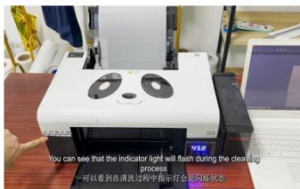
Step 6. During the head cleaning process, the switch button will keep flashing.
