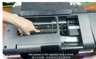
Step 16. Next we're going to add lubricating oil to the guide rail. This should be done once a month.
