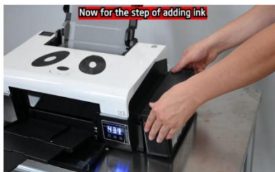
Step 13. Put the ink tank flat on desk.
