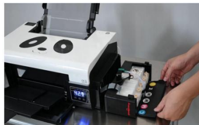
Step 14. Open the tank cover. And pay attention to the ink color labels. C refers to cyan ink, M refers to magenta ink, Y refers to yellow ink, K refers to black ink and W refers to white ink
