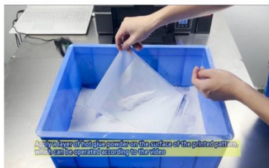
Step 14. Get the printed film. With printing face down, spread the powder on the back of the printing film. Make sure the powder are spread evenly.
