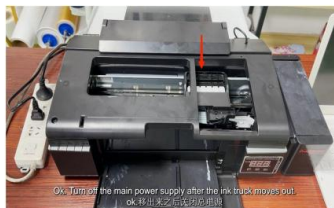
Step 18. When the print head assembly moves out a little, cut down the printer power.
