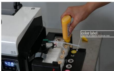
Step 15. Add corresponding inks into these containers. Attention that the max tank capacity of each color is 80ml.
