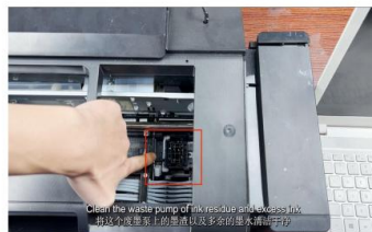
Step 23. Carefully clean the waste pump to remove all the ink residues. Attention not to touch the silicone sealing around.
