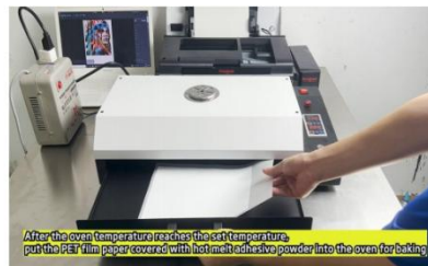
Step 18. With printing film face down, gently put the film on the oven pad. And start the curing.
