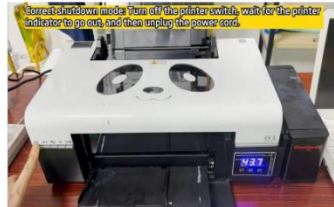
Step 32. Every time after you finish using the printer, long press the switch button to turn the printer off.
