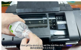
Step 14. Dip lint-free cloth with alcohol.
