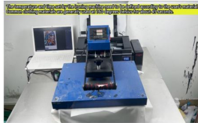
Step 24. Set the heat pressing machine with 160 °C working temperature and 45s pressing time, then close the machine lid.
