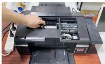
Step 19. Gently drag or push the print head assembly.
