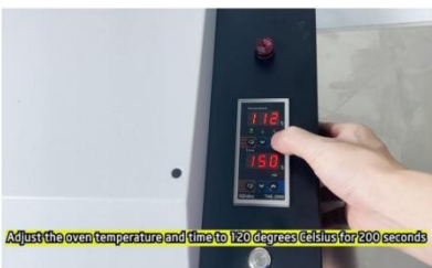
Step 17. To cure the printing film, set the oven with curing temperature 120°C and curing time 200s.
