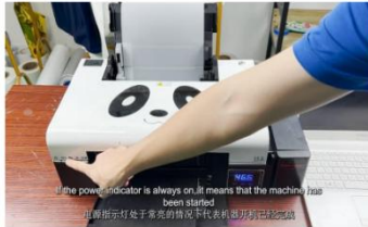
Step 1. Turn the printer on. If the switch button stays on without flashing, that means the machine is ready for any operation.
