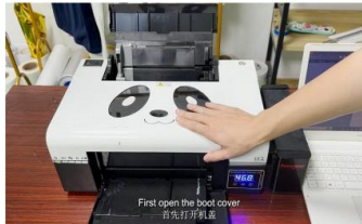
Step 12. Then we go on with the manual machine cleaning. First open the top cover.
