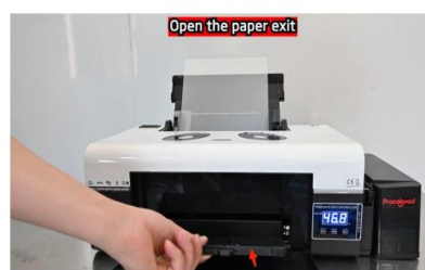
Step 7. Fully elongate the exit tray.
