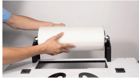
Step 16. Put the film roll onto the bracket. (The printable side with coating facing up)
