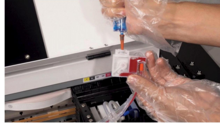
Step 42. Turn it upward to extract 5 to 10ml of ink until there is no much air in the cartridge.
