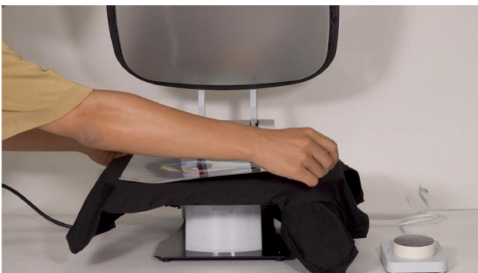
Step 3. Set the temperature of heat press at 135 degrees Celsius and timer to 30 seconds. Put the DTF print onto the T-shirt and start heat transfer. This time, printing face is up.
