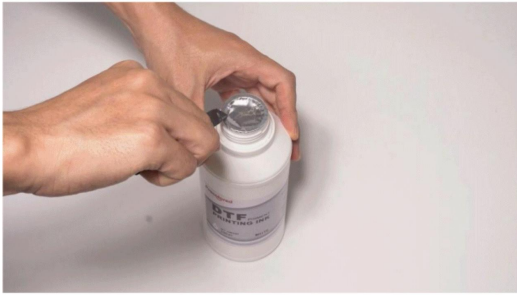
Step 31. Cut off the Aluminum foil seal of the ink bottle.
