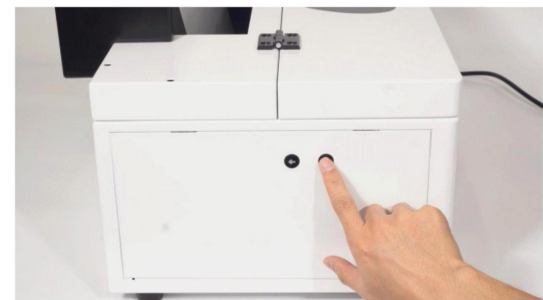
Step 28. Press the forward button to load the printer film.
