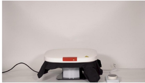
Step 2. Set the temperature of heat press at 135-145 degrees Celsius and timer to 10-15 seconds. This will help get rid of the wrinkles on the T-shirt and iron it flat, so that the pattern on the clothes doesn't absorb uneven pressure.
