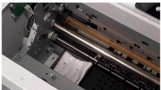
Step 40. Put the ink pad in. This ink pad is to collect ink residue dropping from print heads.
