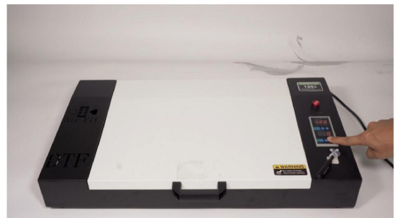
Step 6. When the curing is over, press the button again to stop curing.
