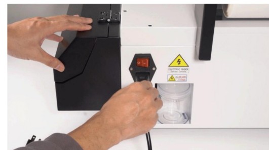
Step 20. Insert the power cable onto printer on its back.
