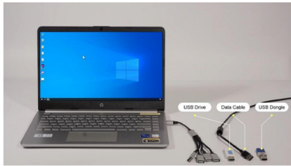
Step 1. Procolored printer can only connect with Windows computer; and we highly recommend you to get a USB hub to simultaneously function different drivers.
