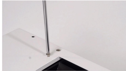
Step 2. There are two screws on each side. Remove the screws.
