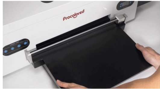
Step 18. Hook the cutter platform at the film exit.
