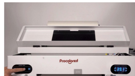
Step 50. Long press the ink button to execute print head cleaning. [the left third button]
