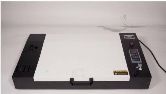
Step 3. Powder curing will be done by an oven like this. Set the temperature at 125 degrees Celsius and the countdown timer to 180 seconds. The curing time is flexible, if the print is too wet, it need longer time to dry up entirely.
