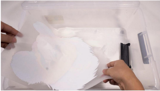
Step 1. Printing face down, spread the powder on the back of the printing film. Make sure the powder is spread evenly.
