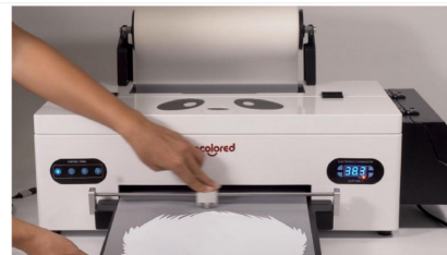
Step 8. Slide the cutter to separate the film and get your printing.
