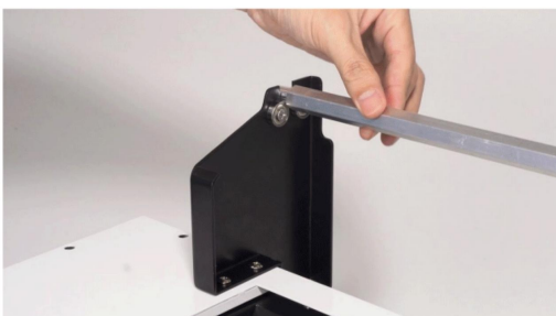
Step 7. Rotate the roller to check if the bracket distance is appropriate and safe.
