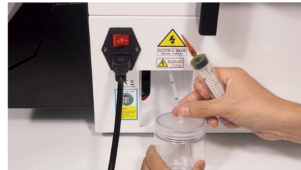
Step 46. Take out the waste ink bottle at the back of the printer.
