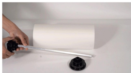
Step 10. Fetch the roller down and slide the plastic holder onto it.
