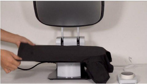
Step 1. Before heat pressing, we need a preheating for the clothes. Put the clothes flat on the pressing pad.
