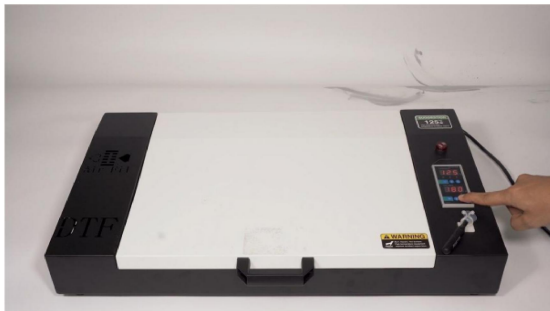
Step 5. Press start and wait for the curing. In the oven, adhesive powder is melting down, inks are curing/drying up and embedding onto the adhesive layer.
