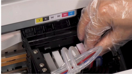
Step 43. Put the cartridge back in place after extracting.
