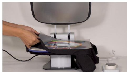
Step 6. When the pressing is over, gently get the clothes off. DO NOT peel off the film right away.
