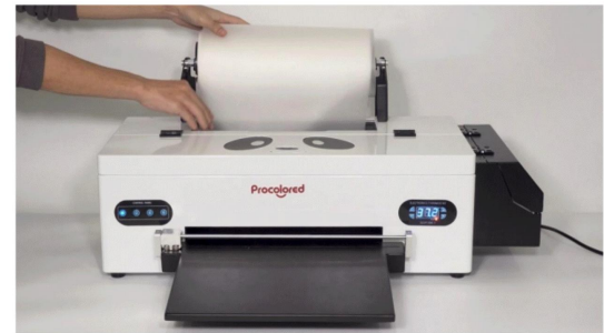
Step 26. Put the film into the film feed under the pickup rollers.
