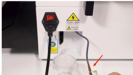
Step 47. Extract 5 to 10 milliliters of ink out of the waste ink tube.
