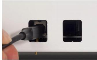
Step 22. Insert the data cable into the left port.
