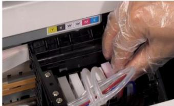
Step 43. Put the cartridge back in place after extracting.
