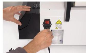
Step 20. Insert the power cable onto printer on its back.
