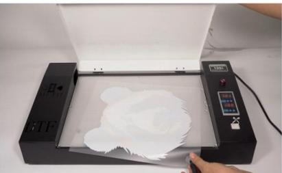
Step 7. We highly recommend to use a suction cup to fetch the cured printing film, since the oven pad and film might be really hot.
