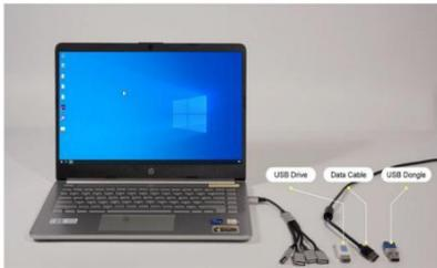
Step 1. Procolored printer can only connect Windows computer, and we highly recommend you to get a USB splitter to simultaneously function different drivers.
