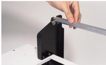
Step 7. Rotate the roller to check if the bracket distance is appropriate and safe.
