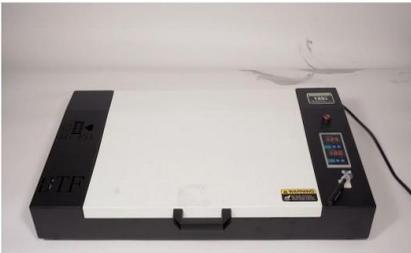
Step 3. Powder curing will be done by an oven like this. Set the temperature at 125 degrees Celsius and the countdown timer to 180 seconds. The curing time is flexible, if the print is too wet, it need longer time to dry up entirely.
