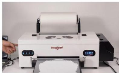
Step 17. When the printing is done, press forward button to load more film.
