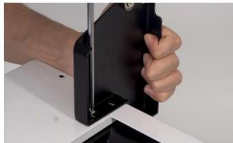
Step 3. Put the bracket on and pay attention to its facing direction. Turn the screws but do not tighten it fully.
