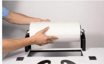
Step 16. Put the film roll onto the bracket. (The printable side with coating facing up)
