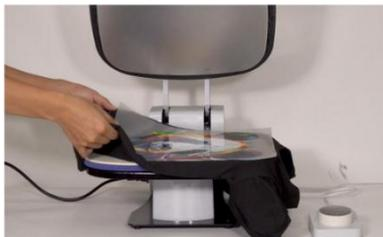
Step 6. When the pressing is over, gently get the clothes off. DO NOT peel off the film right away.
