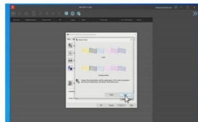
Step 10. You can combine the guidance window on computer to double check the nozzle condition. If there are too many broken lines, clean the print-head again.
