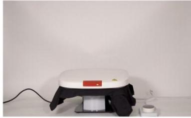
Step 2. Set the temperature of heat press at 135-145 degrees Celsius and timer to 10-15 seconds. This will help get rid of the wrinkles on the T-shirt and iron it flat, so that the pattern on the clothes doesn't absorb uneven pressure.
