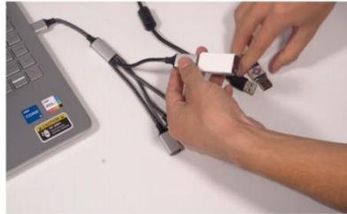
Step 2. Plug the driver, dongle and data cable that Procolored provides into the USB splitter.
