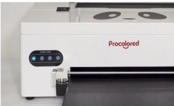
Step 25. The machine is ready when the blue light changes from flashing to always on.
