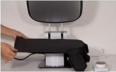
Step 1. Before heat pressing, we need a preheating for the clothes. Put the clothes flat on the pressing pad.
