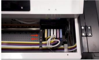
Step 51. The print head will move back and forth automatically to finish the cleaning which takes about 2 minutes.
