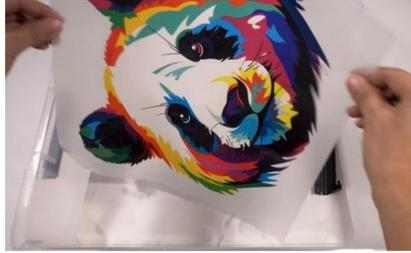
Step 2. Before curing, don't forget to shake the film slightly to remove the spare powder.
