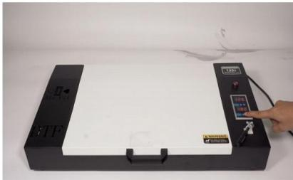
Step 5. Press start and wait for the curing. In the oven, adhesive powder is melting down, inks are curing/drying up and embedding onto the adhesive layer.
