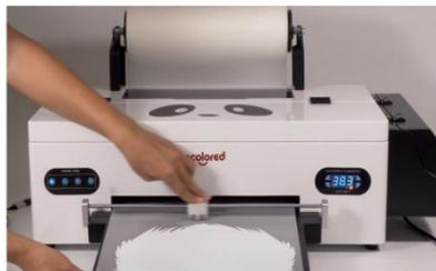
Step 18. Slide the cutter to separate the film and get your printing.
