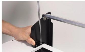
Step 8. Once the bracket position is confirmed, tighten the screws fully this time.
