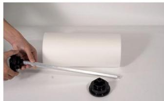
Step 10. Fetch the roller down and slide the plastic holder onto it.
