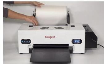
Step 26. Put the film into the film feed under the pickup rollers.
