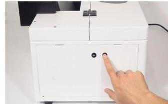
Step 28. Press the forward button to load the printer film.
