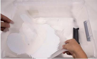
Step 1. Printing face down, spread the powder on the back of the printing film. Make sure the powder is spread evenly.
