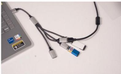
Step 3. Make sure all of them are inserted. The USB drive stores printer software and tutorials. The USB dongle provides licensed access to the RIP software.
