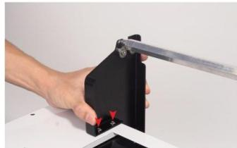
Step 6. Adjust the bracket position to ensure the distance between them can perfectly fit both sides of the roller.
