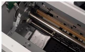
Step 40. Put the ink pad in. This ink pad is to collect ink residue dropping from print heads.
