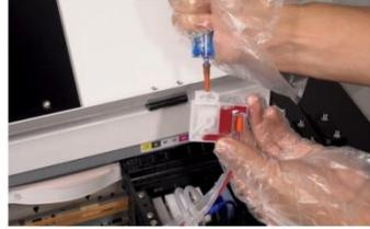
Step 42. Turn it upward to extract 5 to 10ml of ink until there is no much air in the cartridge.
