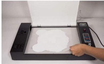
Step 4. Printing film face down, gently put the film on the oven pad.
