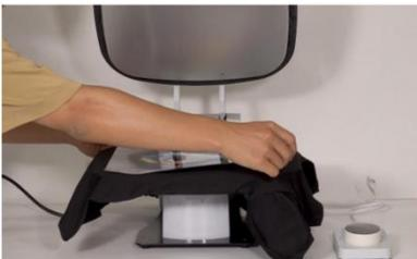
Step 3. Set the temperature of heat press at 135 degrees Celsius and timer to 30 seconds. Put the DTF print onto the T-shirt and start heat transfer. This time, printing face is up.
