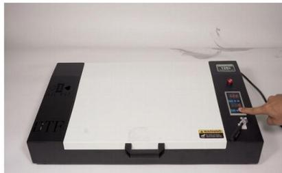
Step 6. When the curing is over, press the button again to stop curing.
