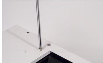
Step 2. There are two screws on each side. Remove the screws.
