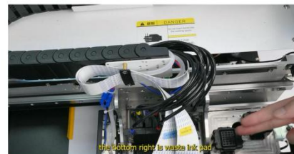
Step 10. check the waste ink pad, right side to collect white ink and varnish, left side to collect colorful ink
