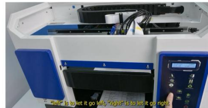
Step 8. Two buttons, "left" and "right", control the print head to move left and right
