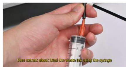
Step 8. Manual extraction of waste ink
