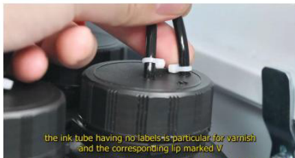
Step 3. the ink tube having no labels is particular for varnish and the corresponding lip marked V
