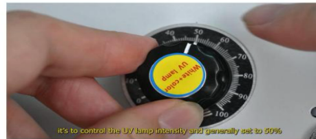
Step 12. it's to control the Uv lamp intensity and generally set to 50%
