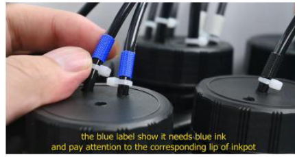
Step 2. Distinguish ink bottles of different colors based on the color of the label on the ink tube
