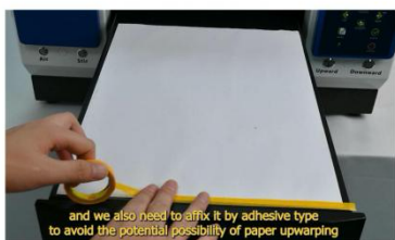
Step 1. Place a piece of white paper on the printing platform and flatten it with adhesive tape
