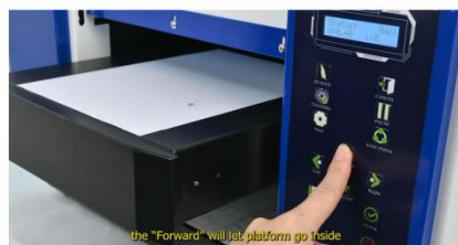
Step 7. Keep press the "Forward" button, it will let the platform go inside
