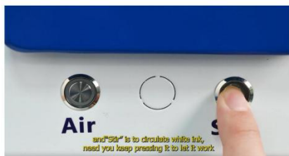
Step 3. Keep press the "still" button to check the white ink cycle operation
