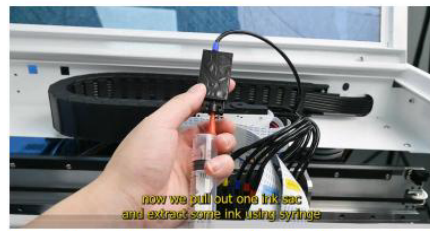
Step 4. Use a syringe to extract 5ml ink from the ink cartridge
