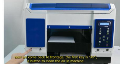
Step 2. Press the "Air" button on the left panel to clear the air from the printer
