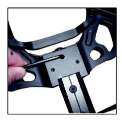
**Step 5:** Attach quiver mount found in the quiver mount hardware packet to the underside of the riser using the 2 counter sink Allen screws provided in the quiver hardware packet as pictured.
