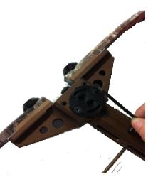
**Step 4:** Insert Foot stirrup into riser. With the crossbow still flipped over insert the foot stirrup into the riser with the two notched areas facing toward the grub screws shown below being tightened. The grub screws may need to be loosened slightly to be able to properly insert the foot stirrup.
