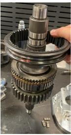
2.4. The detent pieces are bidirectional so there is no right side up to installing them. If the bronze synchro is rotated, a notch can be found where there is a gab in the synchro teeth. Align this notch and gab with the seat for the detent.
