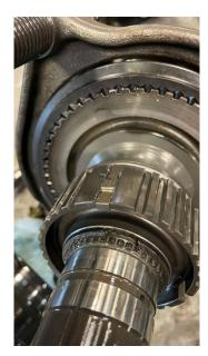
1.6. **IMPORTANT**: The spring rings sitting in the Shift Collar Alignment have a substantial gap. Make sure that the ring is aligned with the three detents so that each detent is spring loaded. If this is not completed, there is a risk that the detent could dislodge itself and damage the internals of the transfer case. Be sure to check the back side ring as well.
