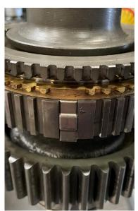
2.6. The shift collar **IS DIRECTIONAL**. One side has teeth that are pointed and the other has teeth that are flat. Face the pointed teeth up (or away from the flange side of the shaft).
