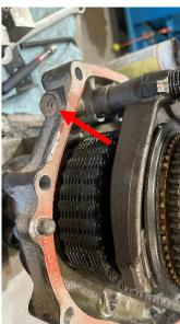
2.2. Remove the rear output flange and bearing retainer. Remove the rear output bearing snap ring and pull the output assembly from the transfer case housing.
