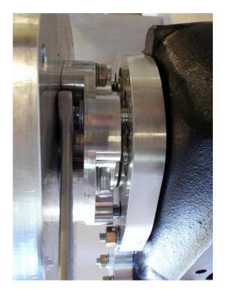
There is enough room to get a box head 5/8" wrench in to turn the cap screw about a third of a turn. Again tighten in a manner to ensure the threads go in strait, after a couple of turns of the wrench, alternate bolts until tight.
