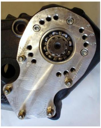
Also install the (8) black socket set screws into what are going to be your unused clocking holes. That is, if you already determined you are going to clock with hole B, thread into all A and C.
