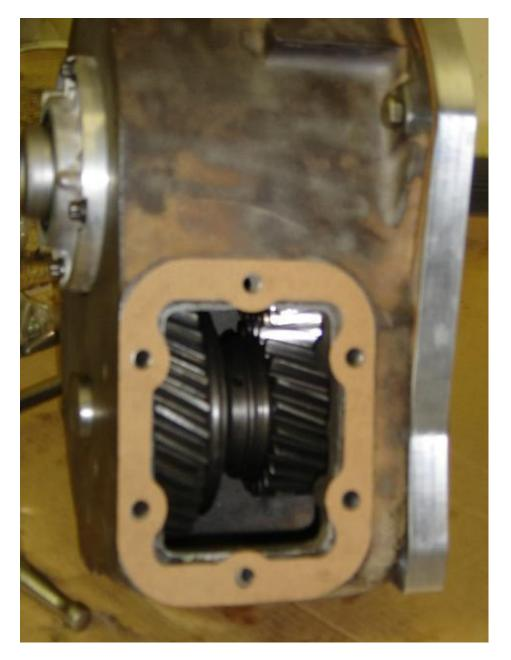
After allowing the sealant to tack, apply another thin coat to the backside of the paper gasket.
