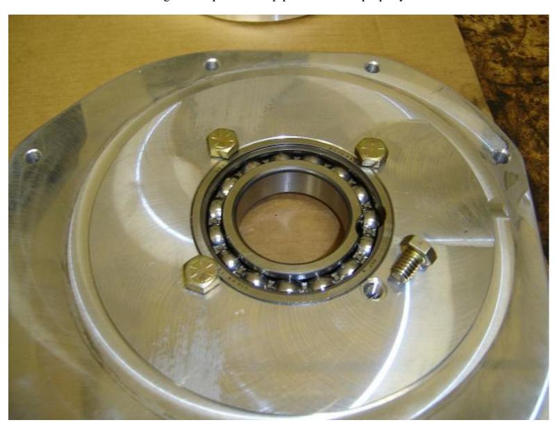
Secure the bearing into place with four 3/8"NC x 1/2" cap screws and four 3/8" Lock Washers (included). Apply Lock-Tite to the threads.
