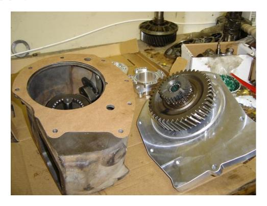
After allowing the sealant to tack, apply another thin coat to the backside of the paper gasket.
