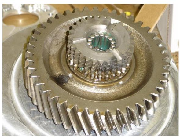
Carefully install the 15 needles so that they 'stick' to the main shaft housing using lots of bearing grease. Assure the bearing grease is clean and no dirt or grit exists.
