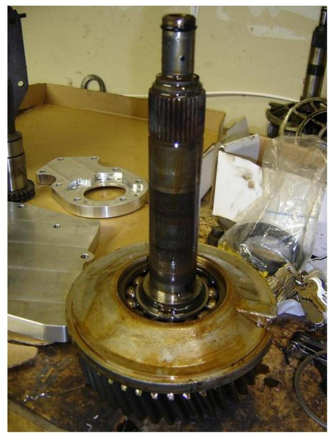
Remove the low range gear and intermediate shaft assembly by pulling it straight out of the range box, and place the assembly on the workbench.
