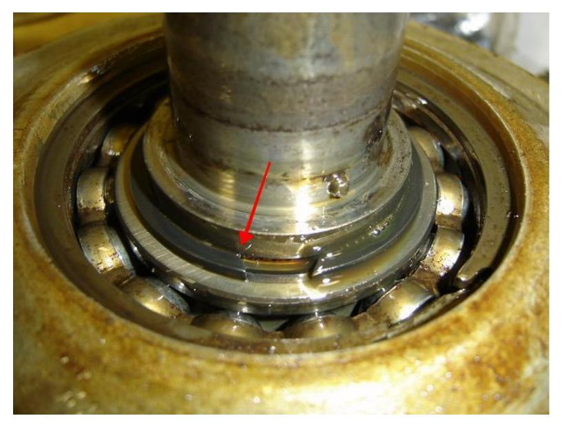
This is accomplished by removing the snap ring retaining the bearing to the shaft. You will need a LARGE set of snap ring pliers. Do NOT use small snap ring pliers; you will snap them and injure yourself in the process.
