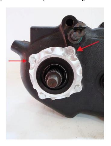
Position the Retainer mount over the NP205 Output as shown, and secure it in place with 3/8" x 1" NC Cap Screws.
