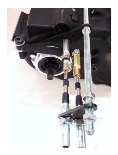
Use the 3/8"x1 1/4" cap screw, (3) 3/8" Nylon washers, and a 3/8" NC Stover nut to join the clevis yoke to the rocker arm.
