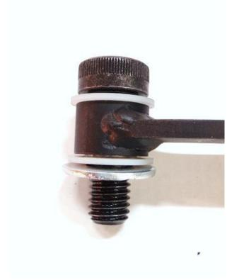
...and thread into the front retainer plate installed in step 1.
