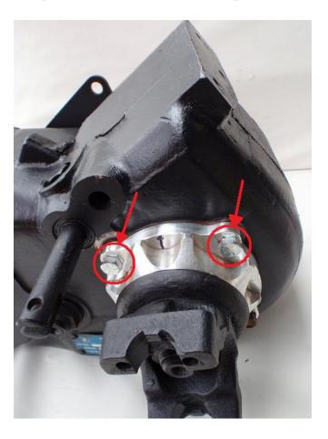
Slide the front retainer plate over the shift rails and secure it to the case with (2) supplied 3/8" x 1" Cap Screw.
