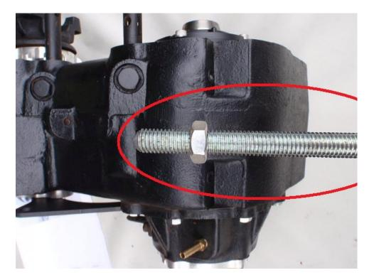
From the output side of the 205 – slide the rod through the top hole of the rear mount installed in step 1. Now thread on 2 more jam nuts and slide the rod through the retaining plate. Thread on one more jam nut and secure rod in place.
