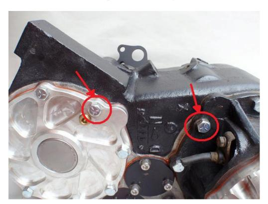
Position the rear mount plate (triangular shape with 3 holes) over the rear of the 205 as shown, and secure it to the case with supplied 3/8" x 1" NC Cap Screws.
