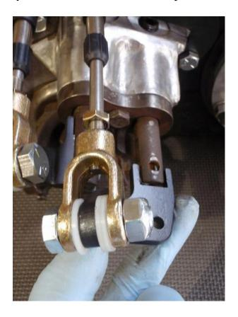
... And fasten with a 1/4 x 1" cap screw and top-lock nut. Lastly tighten cable jam nuts against each clevis.
