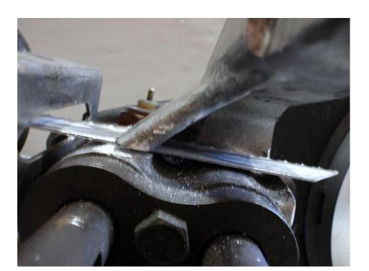
After cutting off the tabs, clean the retainer which encloses the shift rails. We accomplished this with the use of a die grinder and a blending disk.
