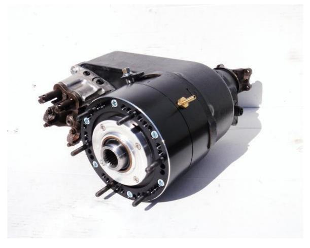
Thread the short coarse thread into the BlackBox-i by first locking two 3/8" NC nuts together on the stud, and turning the top nut with either a 9/16" wrench or socket.
