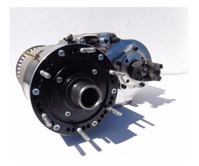
Thread the short side of the stud into the BlackBox-i by first locking two 3/8" NC nuts together on the long side of the stud, and turning the top nut with either a 9/16" wrench or socket.
