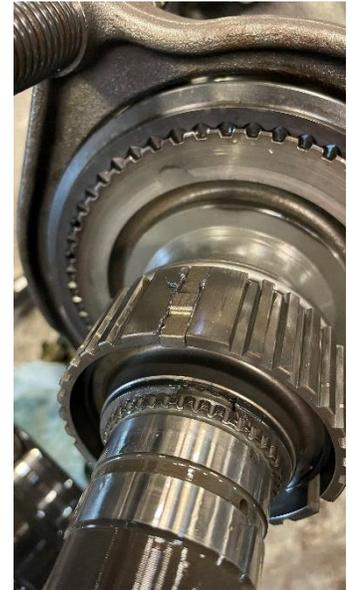
2.1.24 **IMPORTANT:** The spring rings sitting in the Shift Collar Alignment have a substantial gap. Make sure that the ring is aligned with the three detents so that each detent is spring loaded. If this is not completed, there is a risk that the detent could dislodge itself and damage the internals of the transfer case. Be sure to check the back side ring as well
