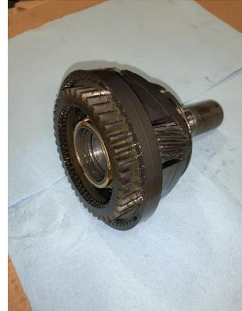
2.1.8 Remove the synchro from the shaft if it hasn't already fallen off. Remove the snap ring holding the low gear engagement and remove the low gear engagement.
