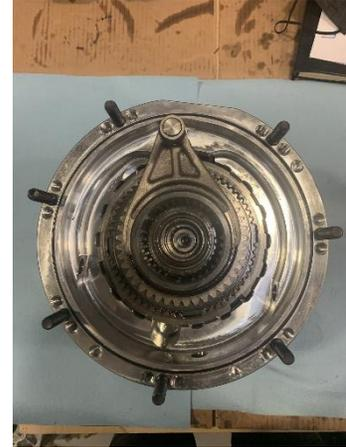
NOTE: The M10 studs define the amount of clocking. The threaded holes on the Lid are spaced by 6° and the clearance holes on the Base are spaced by 10°. This gives a clocking range of 0°, 4°, 6°, 10°, and 16° in the clockwise or counter clockwise direction. The diagram below gives the stud location angles.
