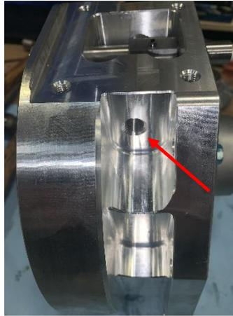
2.2.18 Place the remaining five M8 studs on the transmission. The Eco Crawler and transfer case build is now complete.
