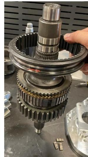
2.1.30 The detent pieces are bidirectional so there is no right side up to installing them. If the bronze synchro is rotated, a notch can be found where there is a gap in the synchro teeth. Align this notch and gap with the seat for the detent.
