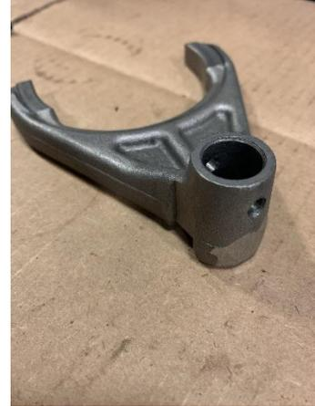
2.2.11 Place the shift collar and the shift fork and install the shift fork and collar into the Eco Crawler. Align the shift fork and rail roll pin holes and press a roll pin in to lock it in place. Make sure that the roll pin is flush with the top of the shift fork.
