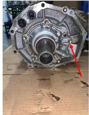
2.1.7 Remove the bearing snap ring. The planetary gearset can now be pulled from the transfer case.
