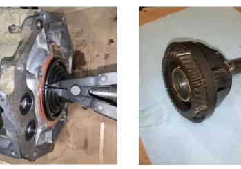
2.1.8 Remove the synchro from the shaft if it hasn't already fallen off. Remove the snap ring holding the low gear engagement and remove the low gear engagement.
