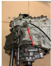
2.1.4 Remove the twelve 12mm or 14mm case bolts. Use a chisel and hammer to work two opposite the case open. The front section of the case is seen on the left of the photo below, this contains the planetary gearset. The rear section of the case is seen on the right in the photo below and contains the rear output shaft, shift fork and shift collar. Set the rear section of the case aside, this will not be needed for the shaft install.
