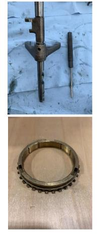
2.2.5 On the rear section of the case, remove the snap ring holding the shift collar alignment. Use a set of jaw pullers to remove the shift collar alignment. Remove the snap rings sitting on each side of the shift collar alignment.
