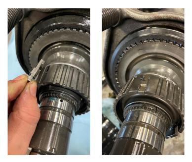
2.1.24 **IMPORTANT**: The spring rings sitting in the Shift Collar Alignment have a substantial gap. Make sure that the ring is aligned with the three detents so that each detent is spring loaded. If this is not completed, there is a risk that the detent could dislodge itself and damage the internals of the transfer case. Be sure to check the back side ring as well
