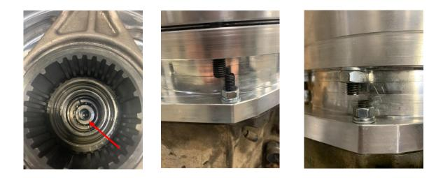
2.2.16 By hand, shift the Eco Crawler from low range to high range. Ensure that the Eco Crawler is fully engaging from low to high. Feel for any points of high friction. If there are points where it feels like the shifting is "sticking" or being held up, open the Eco Crawler case and inspect the shift fork, it will likely need to be ground down for further clearance in step 4.2.10. If the Eco Crawler is not engaging, it could be that the shift fork was placed backwards, refer to step 4.2.11.
