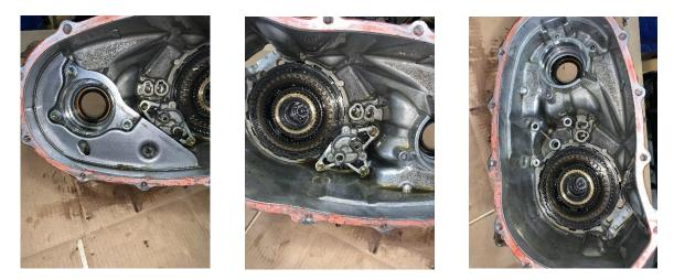
2.1.6 Remove the five M12 bolts that hold the bearing retainer on the front section of the transfer case. Break the silicone seal with a chisel and remove the bearing retainer.
