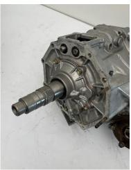
2.1.17 If a **TRIDENT TRIPLE SHIFTER KIT** is being installed on the Eco Crawler and transfer case, the low gear shift rail needs to be ground down for clearance on the double shift legs. Remove the shift fork pin and shift rail detent and pull the shift rail from the rear section of the case. Grind the overhang flush to the clearance surface of the fork on the side and the top, see photos below. Reinstall the rail, the detent and the shift fork roll pin.
