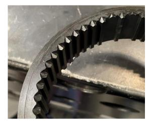
2.1.33 There are gapped sections in the teeth of the shift collar. Align the three spaced teeth with the detent pieces and slide the collar onto the shaft. The detents ride on the spaced teeth with the notch in them.
