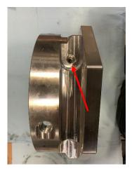
2.2.7 Install the planetary gearset and bearing snap ring. NWF uses a tighter tolerance with the bearing case, this makes the bearing slightly more difficult to press through the bearing bore. Line up the bearing and start the install by hand or until the planetary gear engage with the ring gear. After that, using a deadblow hammer and tapping around the low range engagement will adequately press the gearset into place.
