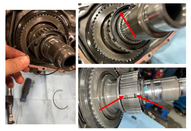
2.1.20 Reinstall the shift collar, shift fork and shift rail. Proceed to step 2.1.27.
