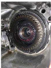
2.1.37 Place the rear section facing up and drop the front section onto the rear. Make sure that the shift rails, rear output shaft and front output shaft are all properly aligned to their respective seats in the front section of the case. If the case does not drop flush to the mating surface, something is improperly aligned. DO NOT force or use an impact gun to pull the case closed. Tap about the case and wiggle it until it falls nicely into place.
