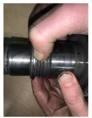
2.1.12 Place the thrust washer, the oil seals, and the split bearing on the NWF shaft. Install the oil seals with the same process as removal but reverse. Be gentle with the seals are they are brittle. It is sometimes easier to install the NWF shaft into the planetary set prior to installing the oil seals.
