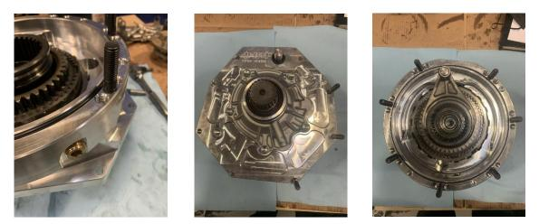
NOTE: The M10 studs define the amount of clocking. The threaded holes on the Lid are spaced by 6° and the clearance holes on the Base are spaced by 10°. This gives a clocking range of 0°, 4°, 6°, 10°, and 16° in the clockwise or counter clockwise direction. The diagram below gives the stud location angles.
