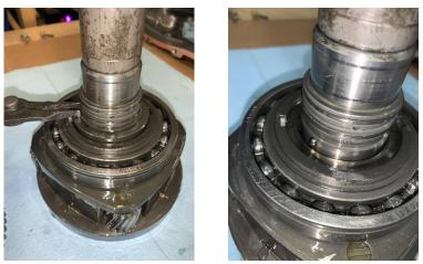
2.1.10 Remove the split bearing from the inside bore of the shaft. The thrust washer for the needle bearing should be stuck to the back of the gear on the shaft. Gently remove it with a flat head screwdriver (If the screwdriver is not catching the lip of the washer, feeler gauges can be used to get underneath the washer and bearing the suction from the oil).
