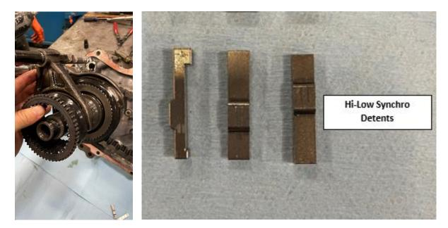
2.1.22 Notice that there are three slots on the Shift Collar Alignment, this is where the three detents sit. There is a spring ring on the front and back of the collar that give the detents the preload to lock in place. Make sure these rings are seated at the inner wall of the alignment piece.
