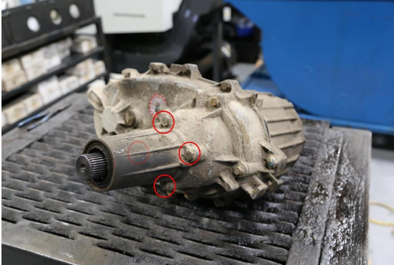
Figure 2: Rear Output Longer Tail Housing Bolts
