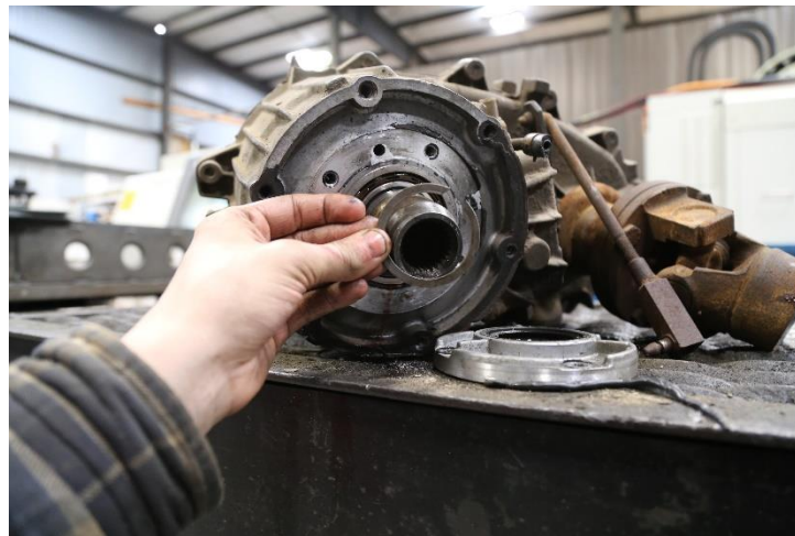
Figure 5: Snap Ring under Bearing Retainer
