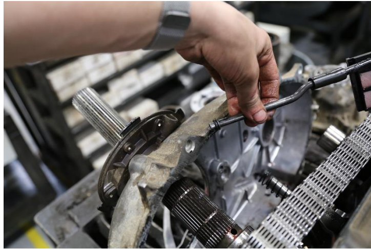
Figure 8: Oil pump connection
