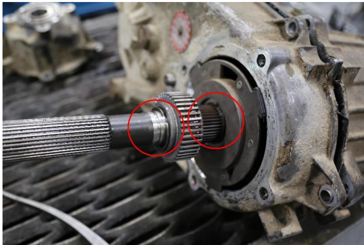
Figure 7: Snap rings around wheel sensor
