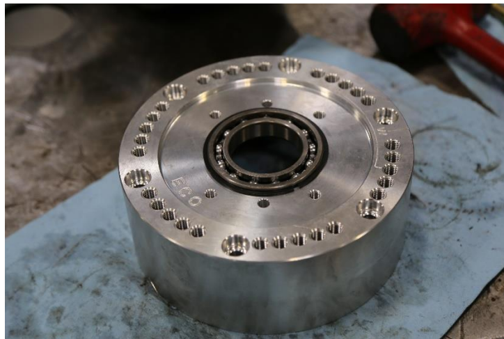
Figure 5: Input bearing pressed into lid
