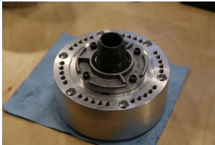
Figure 9: Installed bearing retainer
