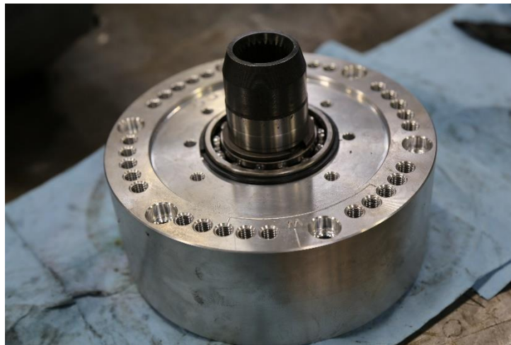
Figure 7: Input shaft seated with snap ring
