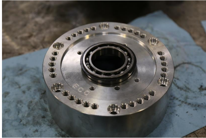
Figure 4: Input bearing placed on lid
