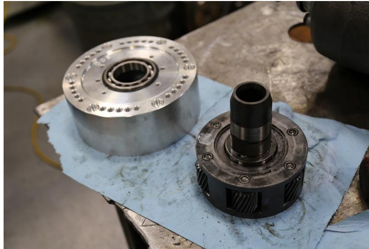
Figure 6: Inserting input shaft and planetary gears
