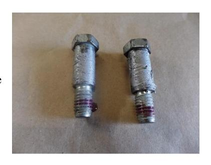
You do not need to use the factory washer when installing the stock shoulder bolts, in fact, there will be a gap between the head of the bolt and the shock eyelet. This is normal. The rear shoulder bolts act as an axle
