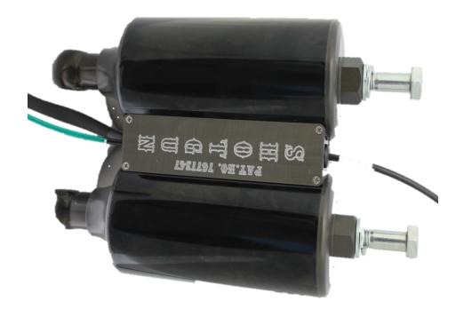
With shock installed trim and install airlines into diverter valve. Be sure not to cut the lines too short, also be sure they do not get pinched or kinked "BLACK" line from front of shock into black 5/32" fitting
