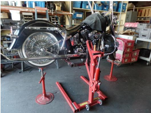
Remove the seat, splash guard, battery and stock shocks.
