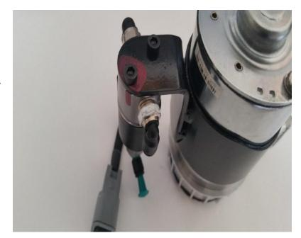
Compressor installed correctly (2007- up non ABS shown)
