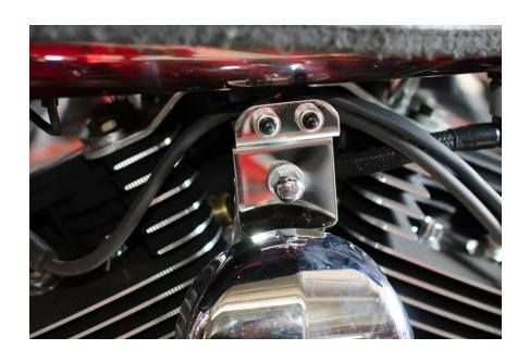
Switches Mount on horn bracket
