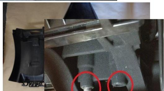
are difficult to break free, use a heat gun at the shock boss)On 2000-2006 models, you will need to tap the existing holes in the bottom of the transmission housing (tap included) in order to mount the compressor.
