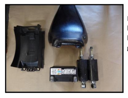
If the stock shoulder bolts are difficult to break free, use a heat gun at the shock boss.
