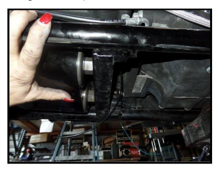
Remove "L" bracket from compressor bracket and attach to Left side bolt
