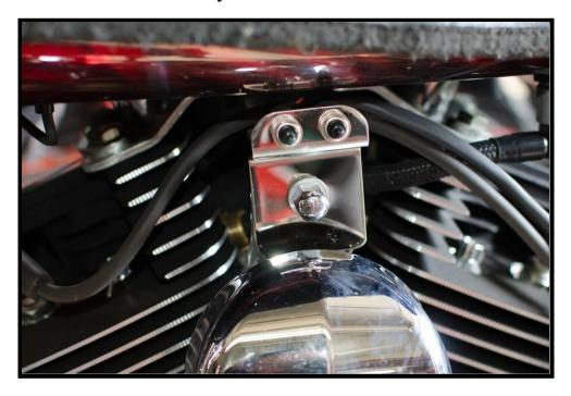
Route switch wiring under tank, and under the ground strap
