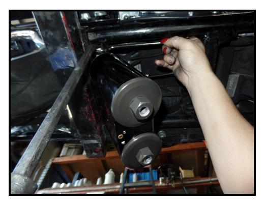
Raise the swingarm, so the shock clears the frame rail
