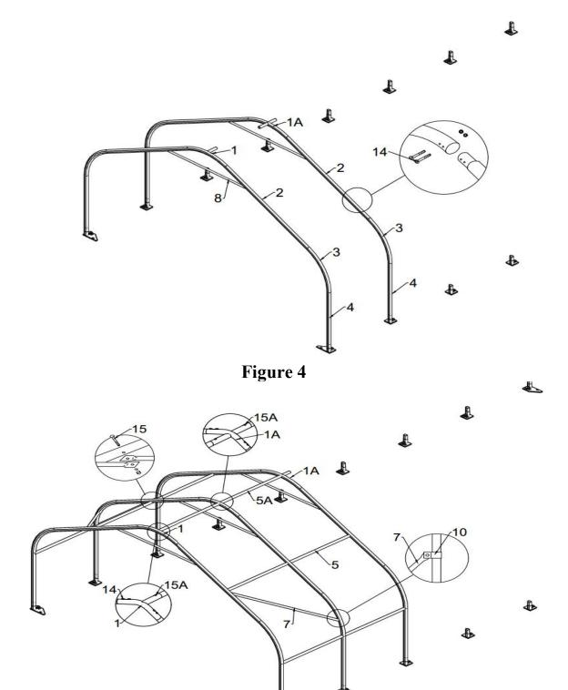
3.4. Assemble middle ribs as shown, Securely fasten all of the joints with the hardware indicated.
